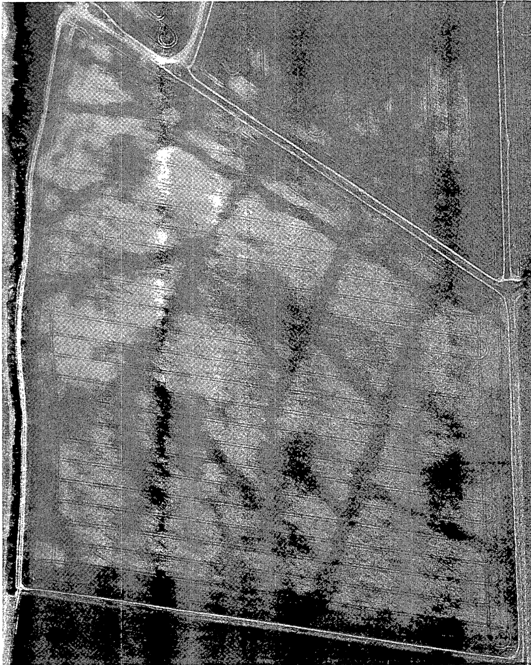
Figure 5. Take-all showing as pale areas in winter wheat on poorly-draining chalky boulder clay where moling had been neglected for the last ten years. The dark lines show better growth over the tile drains. Nuthampstead, Herts., 14 July 1987. (Panchromatic)
